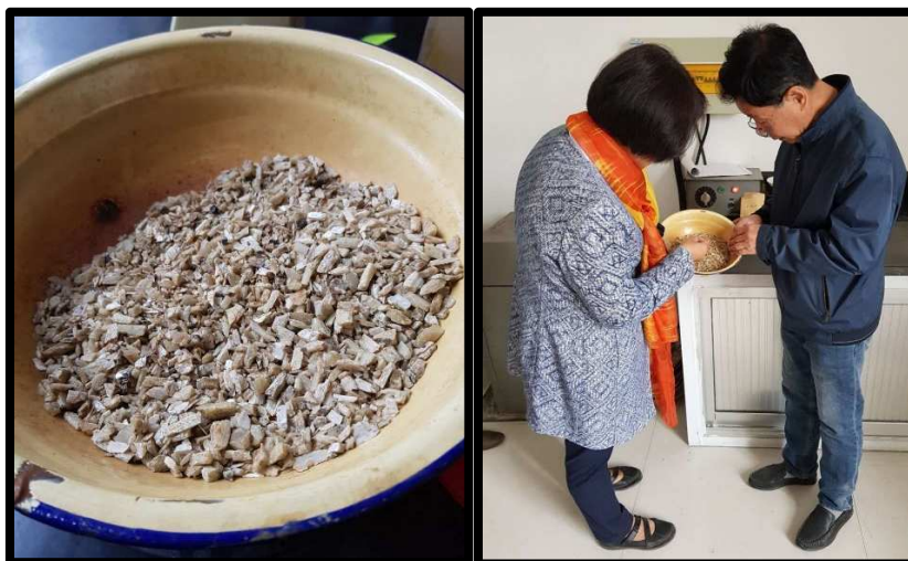
Figure 5. Images of a concentrate produced in 0.5mm to 6mm range (Left), Ardiden Director, Dr. Michelle Li inspecting the sample and discussing the testwork with Prof Gao (Right).
