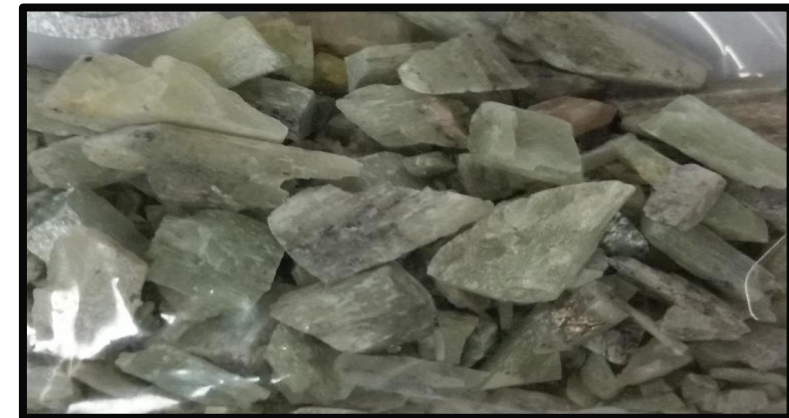
Sample of coarse lithium concentrate (Spodumene) created with DMS at the specific gravity of 3.10 sourced from the Seymour Lake Lithium Project
