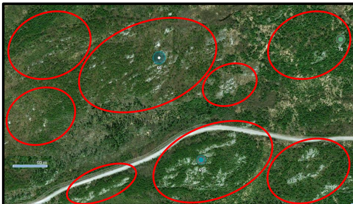
Figure 2. Satellite image of Target area 65, 66 and 70 next to the all-weather road, showing numerous rock exposures that require further investigation to determine if there are any spodumene bearing pegmatites structures.
