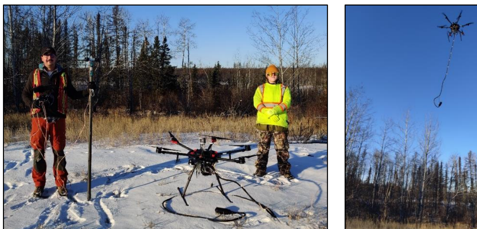
Figure 5- UAV Magnetic Survey Equipment Setup at South Limb
