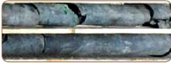
Example of Massive Magnetite from Mariposa Total iron grade: 64% max, 46% average
