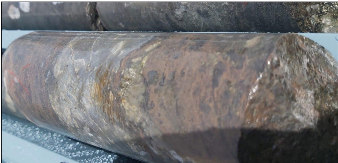
Figure 4: Core photograph of 20cm interval of the upper mineralised zone, semi-massive sphalerite and galena with best result of 2.6% Zn and 1.3% Pb with elevated silver to 41g/t over 0.9m from 139m, A3RCD093.
