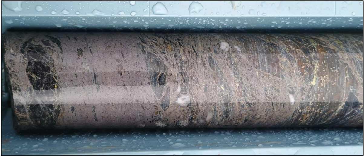
Figure 3: Core photograph from A3RCD094 which returned 0.8m at 310g/t AgEq from 265.3m
