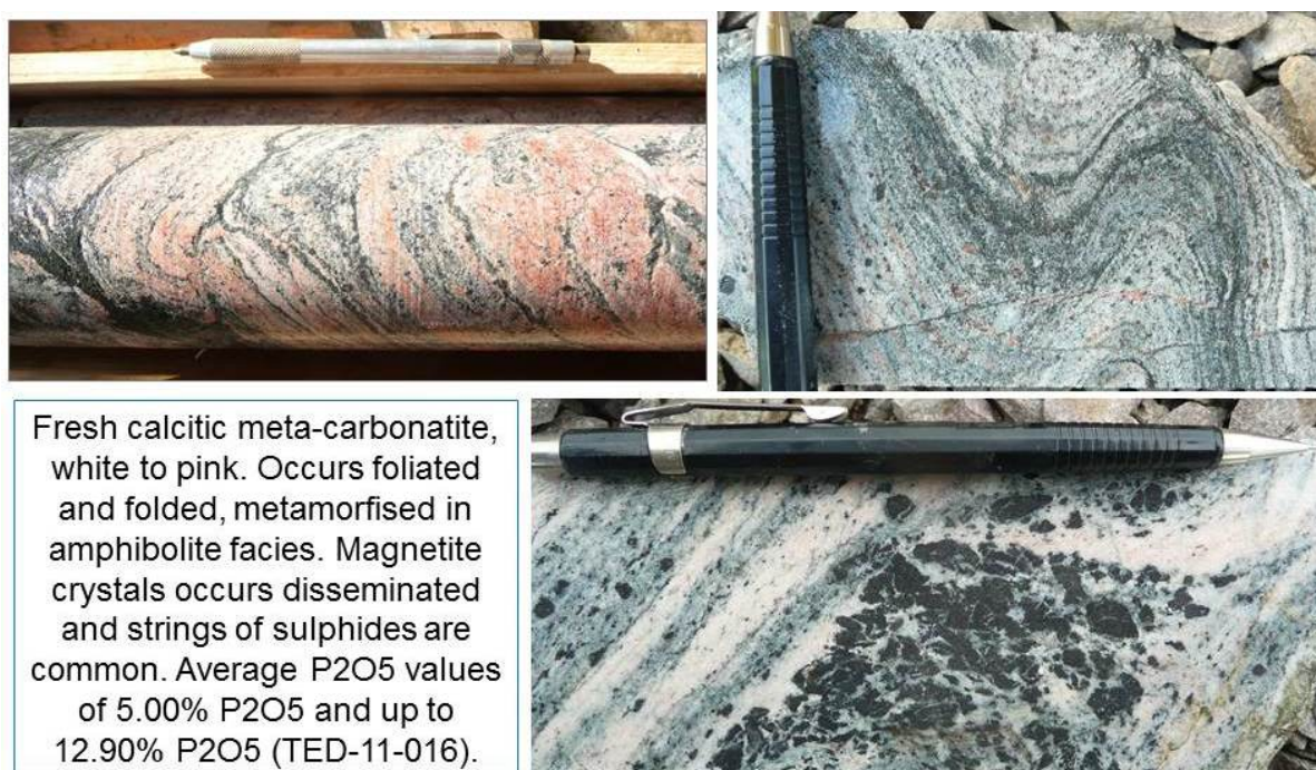
Figure 5: Photos of Fresh (Primary) Meta-Carbonatite Drilling Samples as per Sample EB-02
