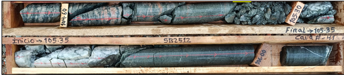
Photo 6 Drill Hole SB-25-12, Vein #1 intersect from 105.1 to 105.75m, showing two stages of quartz, approximately 5% pyrite content, 2% sphalerite and 1% galena, returning 10.3 g/t Au over 0.65m Sample DH020099).
