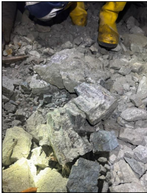
Photo 2: better efficiency in controlling powder factor results in less pulverized material minimizing direct losses
