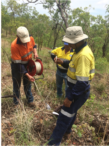
Figure 1 NRC Consultants taking water level readings at MT Porter
