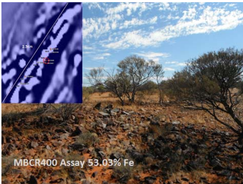
Figure 7. Bonecrusher Sample MBCR400 rock chip assay 53.03% Fe
