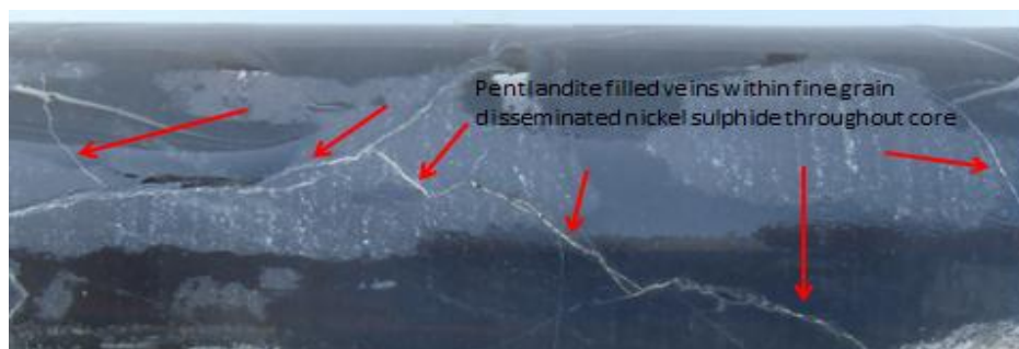
Figure 4 Pentlandite + Pyrrhotite in veins and disseminated sulphides in core from AHDH0006 at 70.4m down hole
