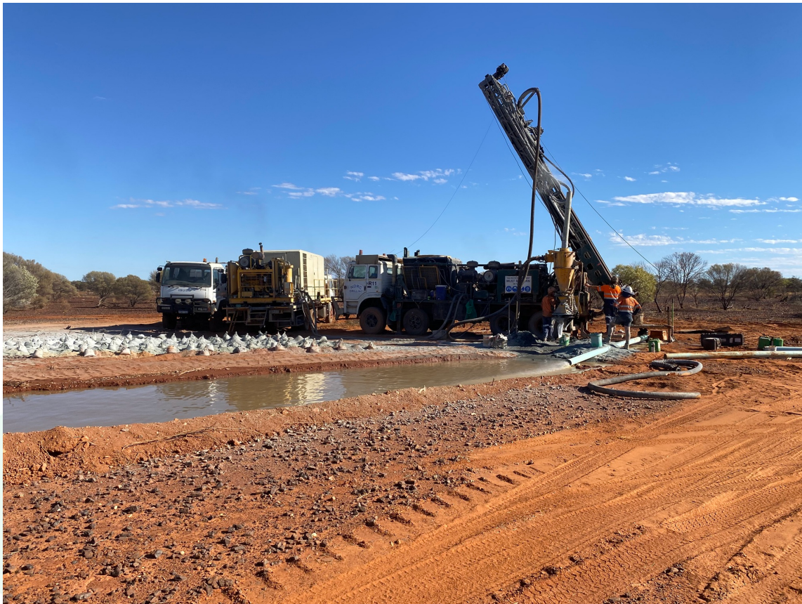
Figure 3: NDRC Pty Ltd reverse circulation rig in action at Byro South
