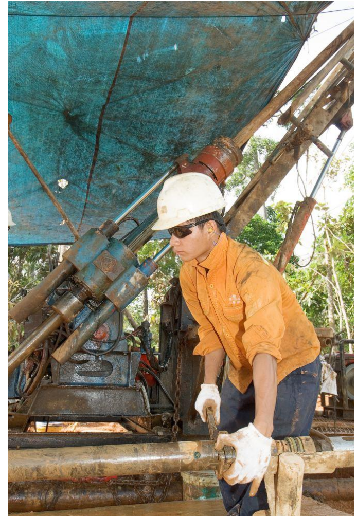
Diamond drilling, Bantian resource drillout
