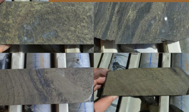
Close up pictures of massive and banded sulphide TKJD008 572 to 578m downhole
