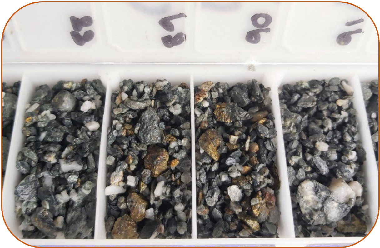
Figure 5: CBLRC027 87 – 91 metres showing vein chalcopyrite-pyrite from 88-90 metres.
