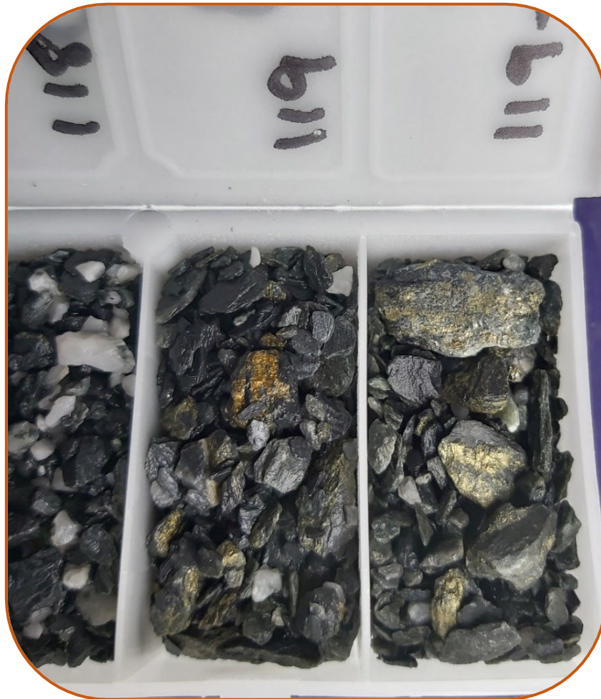
Figure 7: CBLRC026 118 – 120 metres showing vein and stringer chalcopyrite-pyrite.
