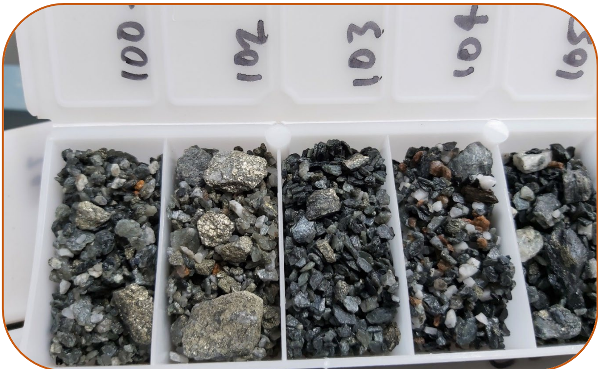
Figure 6: CBLRC024 100 – 105 metres showing vein and semi-massive chalcopyrite-pyrite from 101-102 metres.
