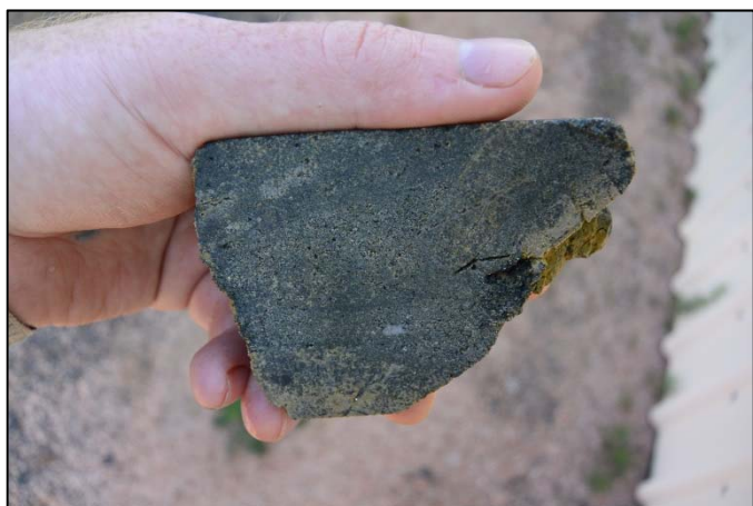
Figure 2. Chalcocite mineralisation replacing pyrite in the supergene enriched copper zone.
