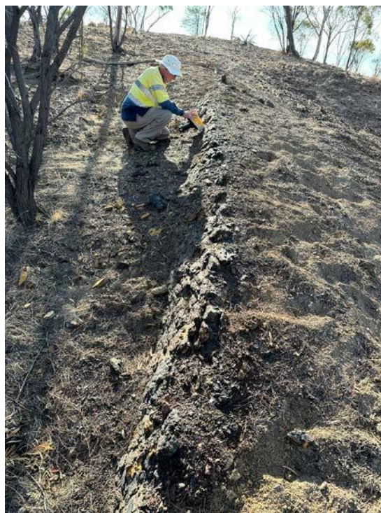
Figure 10. Base Metal Target - Outcropping fine-grained sedimentary rock of the Ronlow Beds with cleavage steeply dipping toward NE - strike NW-SE - yellow-ochre, black & brown limonite possibly derived oxidation of sulphides at depth. The petrology sample collected at this location (GDA2020 343440mE and 7483340mN Zone 55) and shown in Figure 11.
