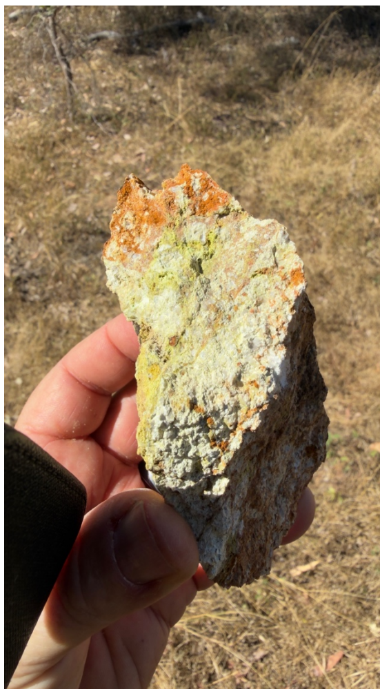
Figure 6. Left EPM 27811 Leichardt Creek LCR 006 3.59g/t Au 5.83% As 184g/t Ag 0.417% Cu, 15.5% Pb and 0.274% Zn Sericite altered metasediment with white secondary Pb minerals and yellow staining after sulphides. Mullock sample.
