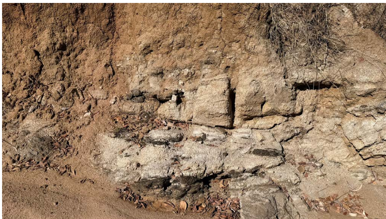
Figure 5. EPM 27811 Leichardt Creek showing granite outcrop in the creek with transported covers up to 2m thickness at the ground surface.
