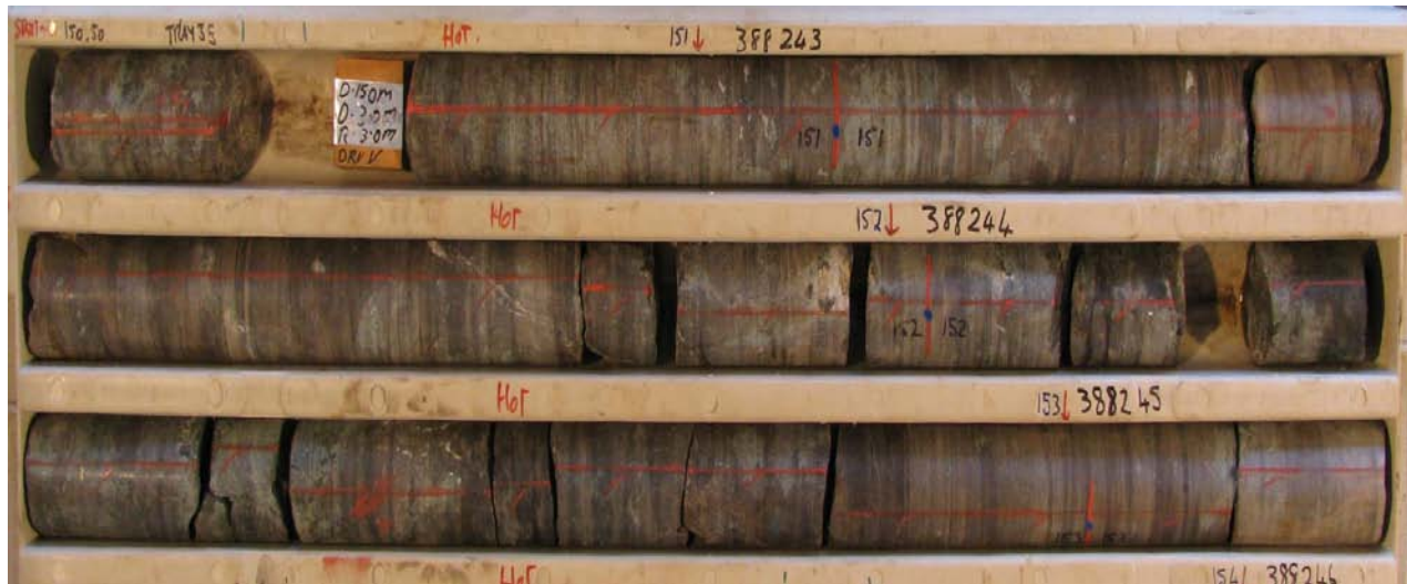
Photo 2: MKED004, ~151.00 to 153.00 metres – REE mineralisation associated with carbonate-magnetite-tremolite alteration. Presence of black mineral laths, tentatively identified as allanite Assays returned for interval = 2m @ 4427ppm TREO and 0.15 kg/t U_3O_8
