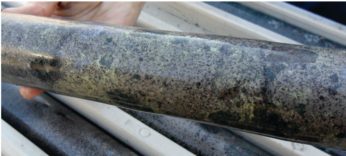
Plate 1. MKED007. Disseminated pyrrhotite - chalcopryite 489 metres (announced previously).
