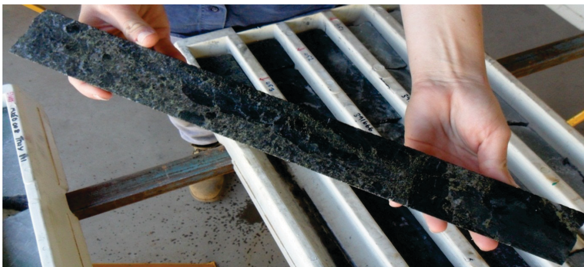
Plate 3. MKED008. Disseminated pyrrhotite (iron sulphide) matrix with disseminated chalcopyrite (copper sulphide) 453 metres.
