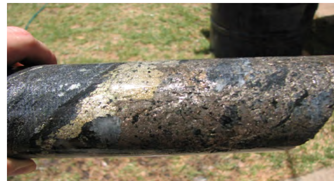
2012 – Diamond drilling – chalcopyrite sulphide mineralisation intersected in core
