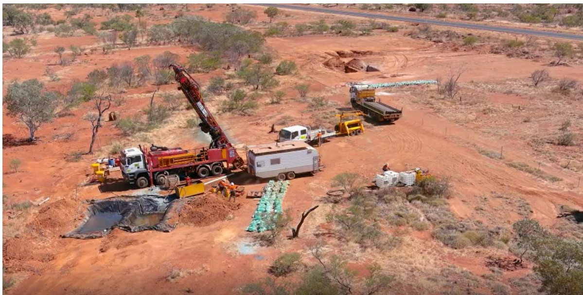
Figure 1 – Diamond drilling at Sandiego
