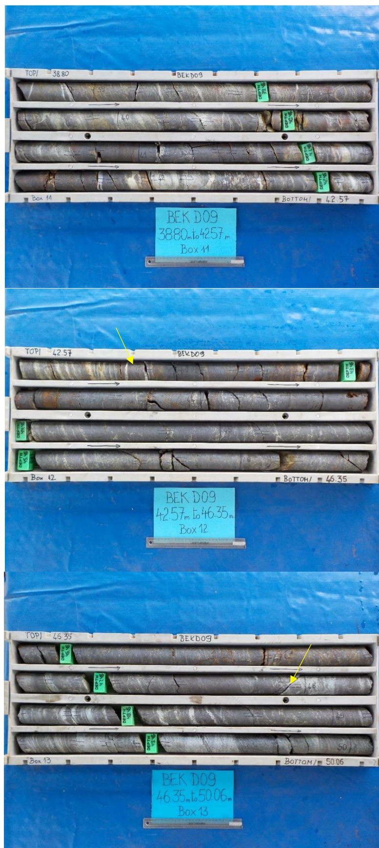
Figure 13 BEKD09; Massive Magnetite mineralisation from 42.8m to 48.0m (yellow arrows mark start and finish) within a zone of more lenticular Magnetite mineralisation
