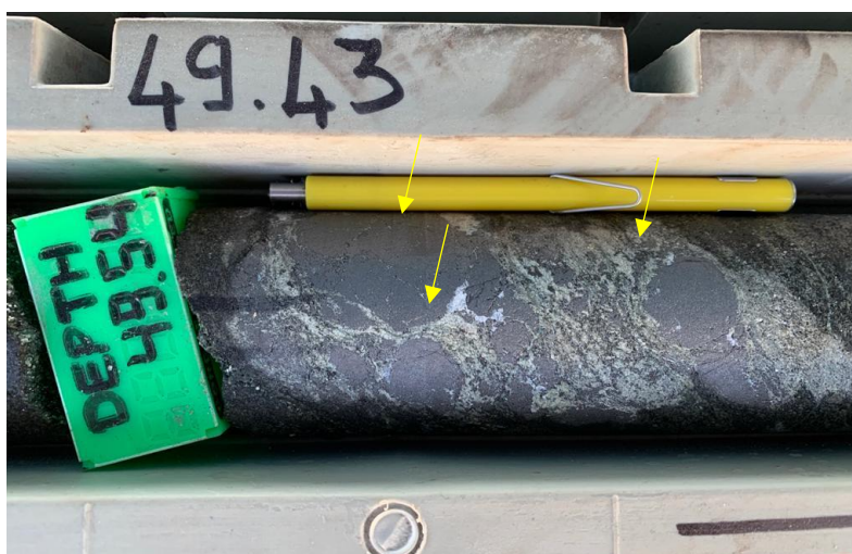
Figure 7 BEKD01 49.5m – Close-up of Pods of Massive Magnetite (black mineral, examples shown with yellow arrows) in Calc-Silicate Host Rock (white and green minerals)
