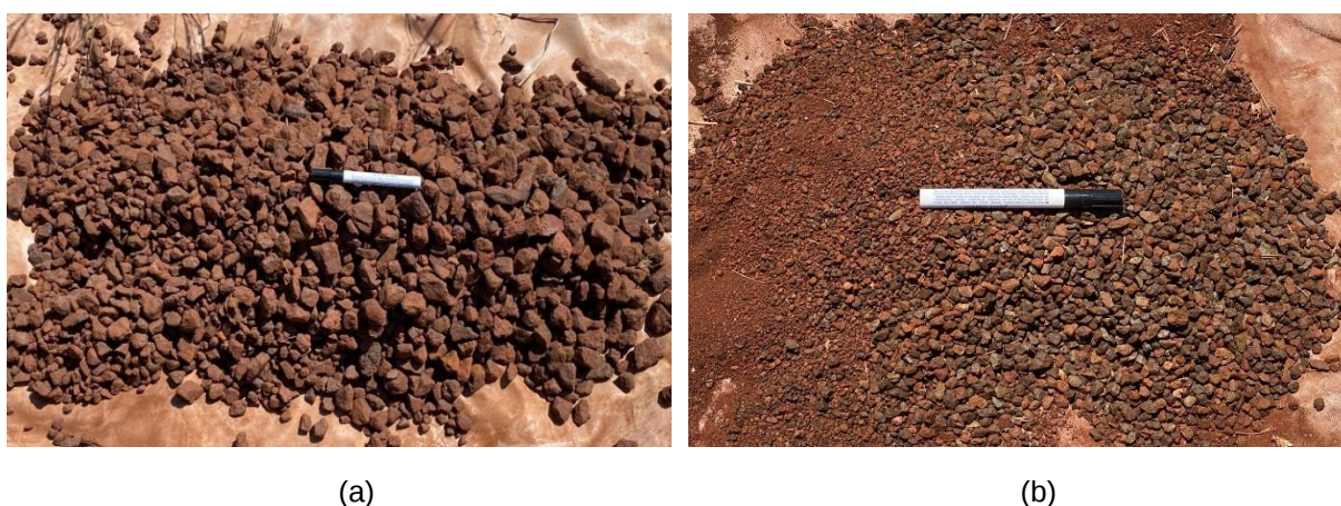
Figure 4. Typical pile of screened bulk samples, lump product (a) and fines product (b)
