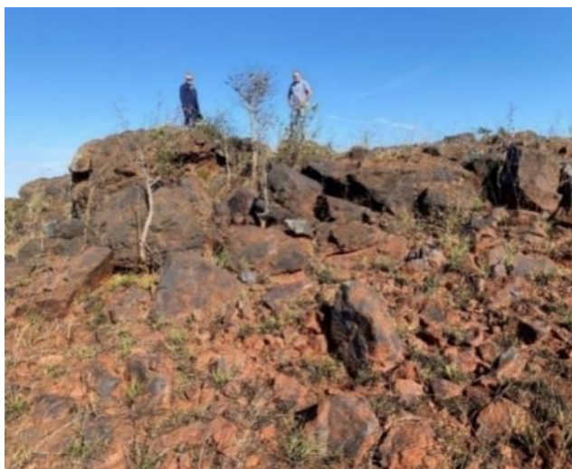
Figure 6a. Massive outcropping iron ore at Bekisopa, rock chip average grade of 66.7% Fe, suitable for lump and fines iron ore products.
