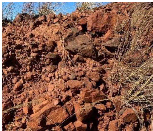
Figure 6b. Iron ore mineralisation in the surface weathered zone, suitable for lump and fines iron ore products.
