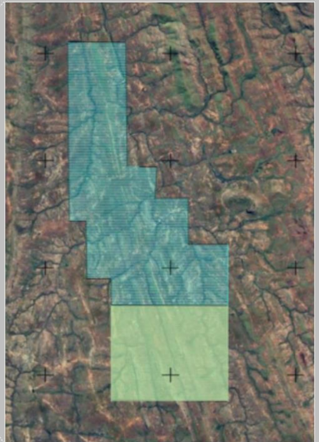
Figure 3. The ground magnetic survey area within Satrokala tenements 27211 and 35827. The Southern area walked on a 25m line spacing, light green area, with the remainder at a 50m line spacing, light blue area.
