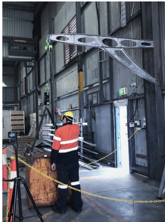
The davit produced through additive manufacturing was comprehensively function tested to twice its design load, by Austal (image: Austal Australia)
