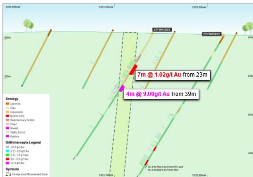
Figure 2: Cross section at Barwidgee Fault Prospect drilling.
