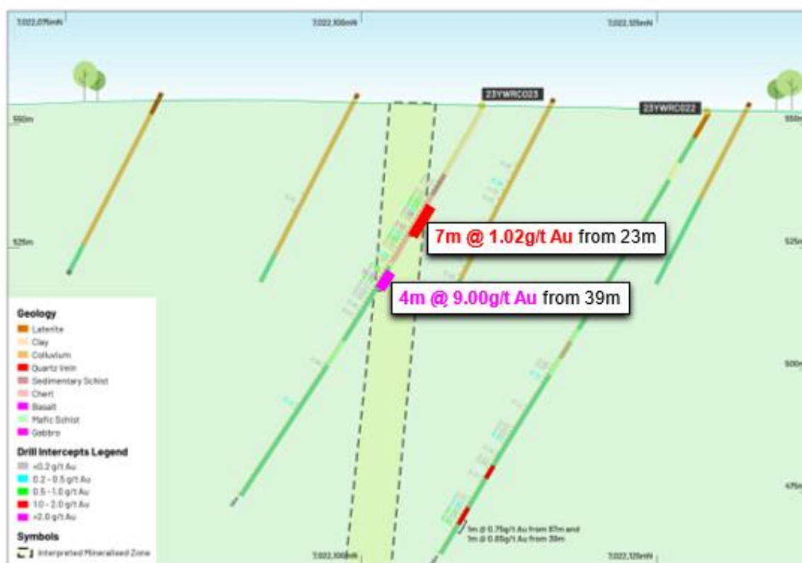
Figure 2: Cross section at Barwidgee Fault Prospect drilling.
