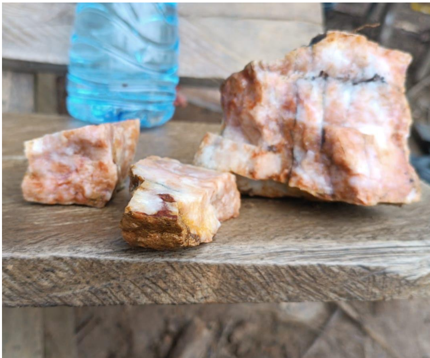
Figure 3: Sheared quartz sub-crop with limonite and dotted pyrite unearthed at the W1 target at 272,459E, 695,607N (WGS84 UTM Zone 21N)
