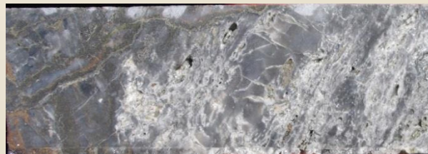
OFDD001: 246m (left) & 248.5m (right) drill core showing strong shearing, epithermal Qtz veining, pyrite (py) & sphalerite (sp)
