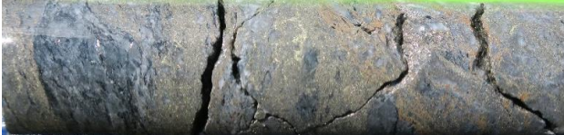
OFDD003: sheared quartz vein with semi-massive pyrite-sphalerite-galena (277.4 - 277.6m)
