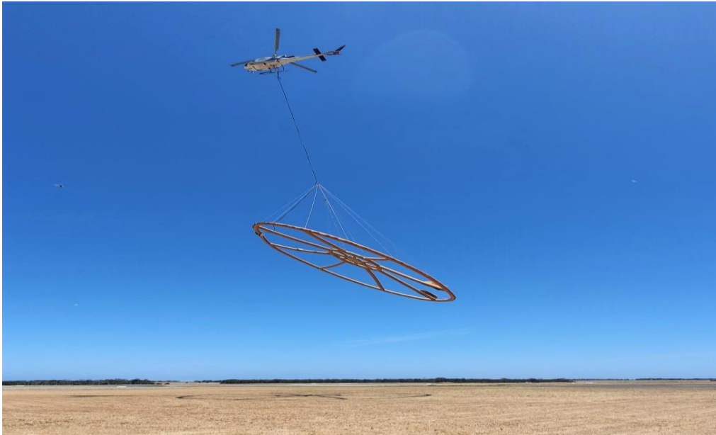
Figure 4. NRG Squirrel helicopter with electromagnetic system on site at Ravensthorpe (January 2022).
