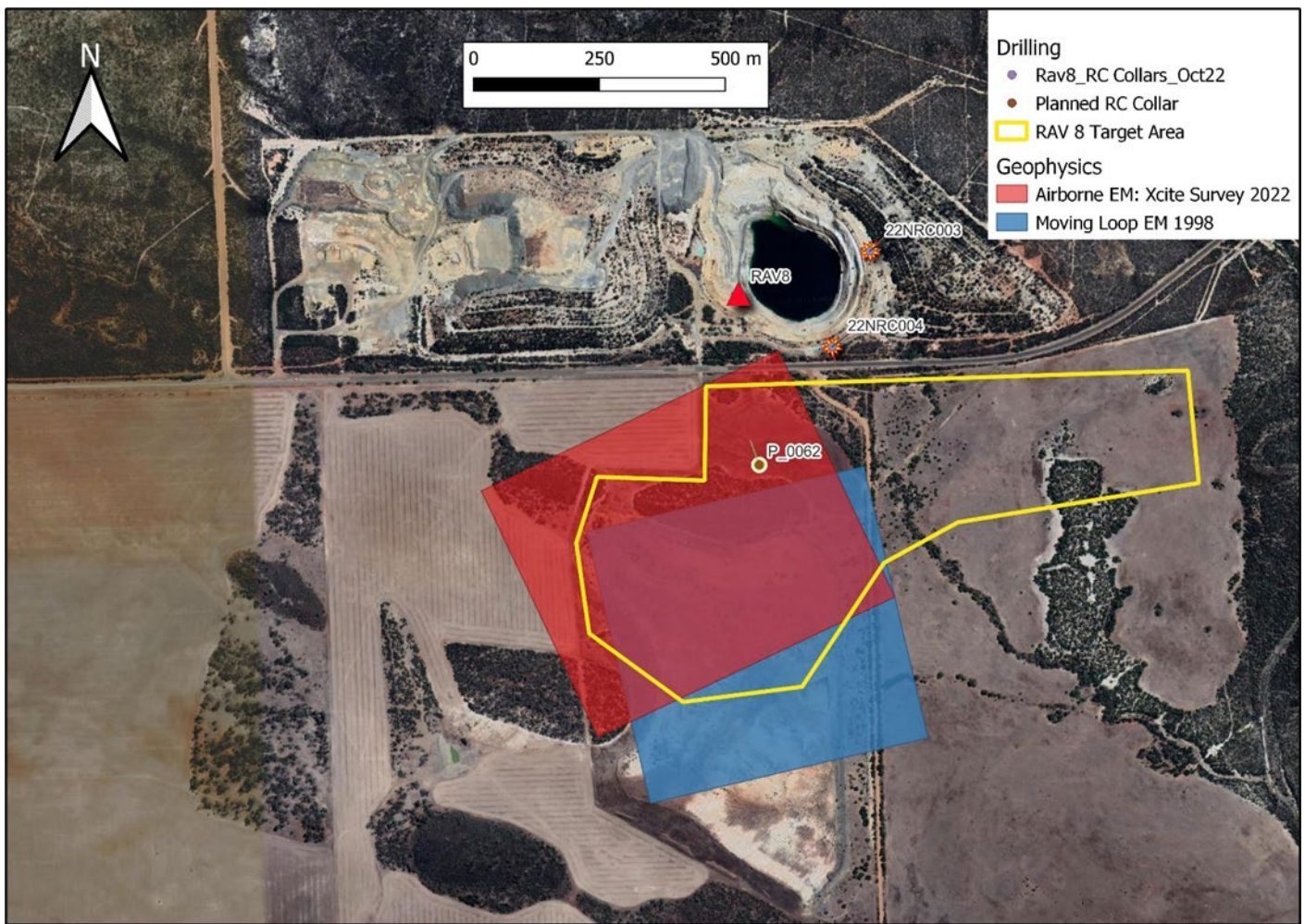
Figure 5: RAV8 South collar location and underlying geophysical plates
