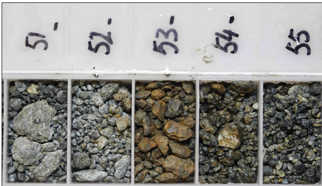
Figure 6: Visually logged chips 51m-55m in 23NRC019 showing abundant disseminated nickel sulphides (brown colouration is due to the sulphides oxidizing) *
