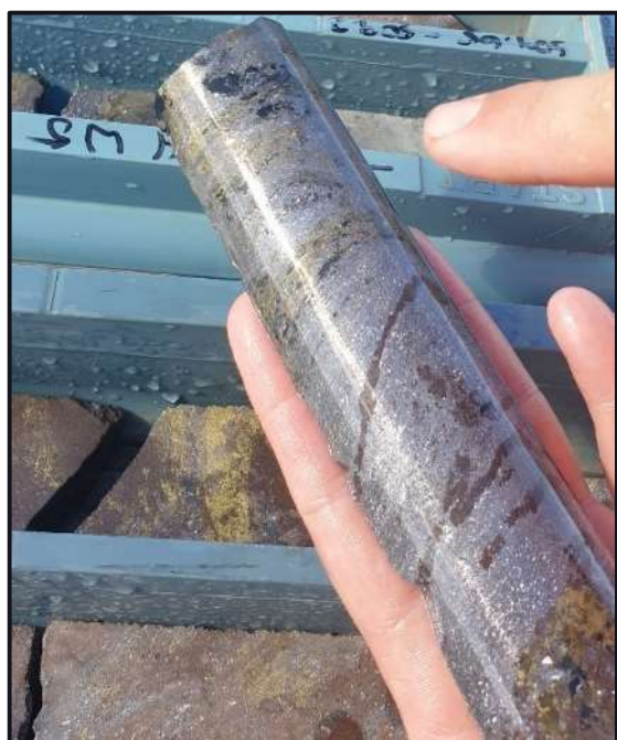
FDD184W5 – 504.4m : Massive sulphides dominated by galena, with strong sphalerite and chalcopyrite, and visible gold
