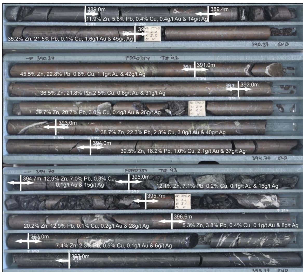
Figure 1: Federation West drill core from drillhole FDR0354, between 388.7m to 398.8m showing significant intersection 9.0m @ 28.3% Zn, 15.4% Pb, 1.2% Cu, 0.9g/t Au and 27g/t Ag from 389.0m including 5.4m @ 39.4% Zn, 21.4% Pb, 1.7% Cu, 1.4g/t Au and 36g/t Ag from 389.4m.
