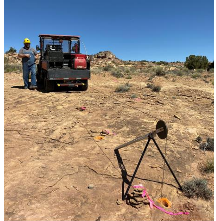
Gamma logging historical drill holes at the Jeffrey project.
