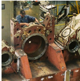
Specialised machining and line boring
