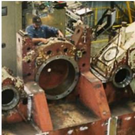
Specialised machining and line boring
