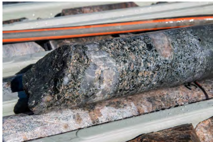
Mineralised zone in EHRCDD003 (329.6 m -329.8 m) – Pyrite dominant with lesser chalcopyrite
