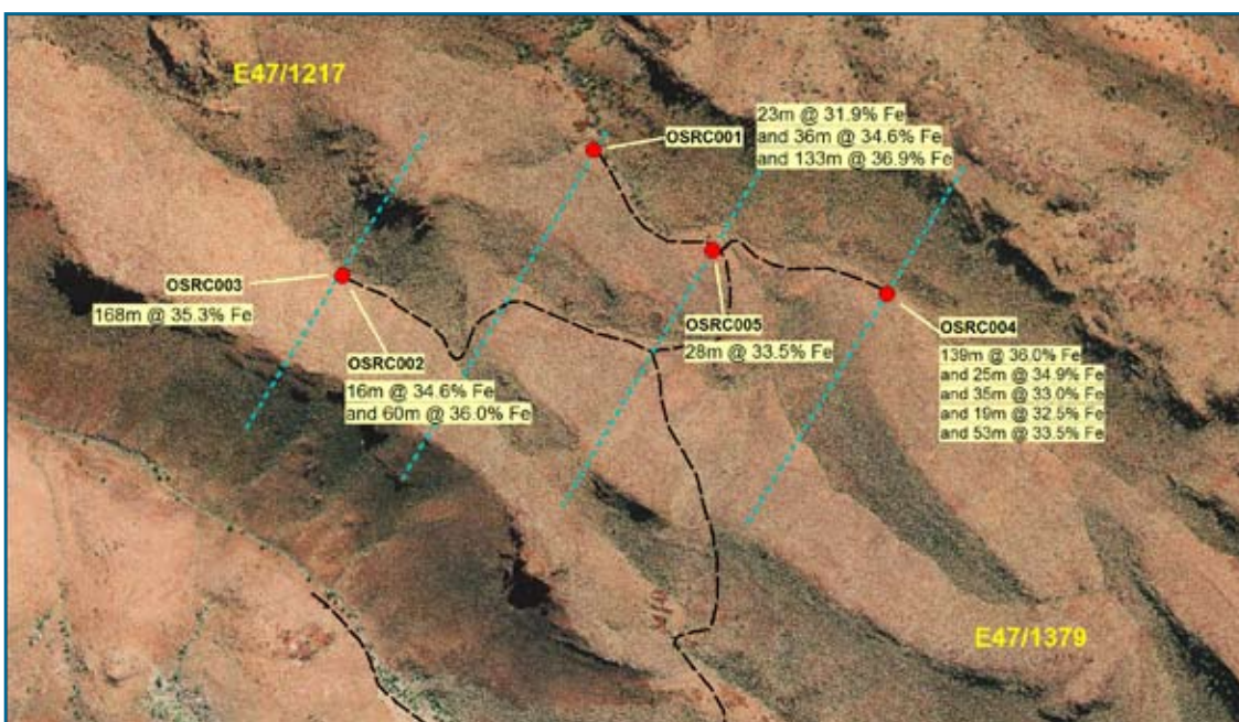
Figure 4: RC drill hole layout and results superimposed on aerial
