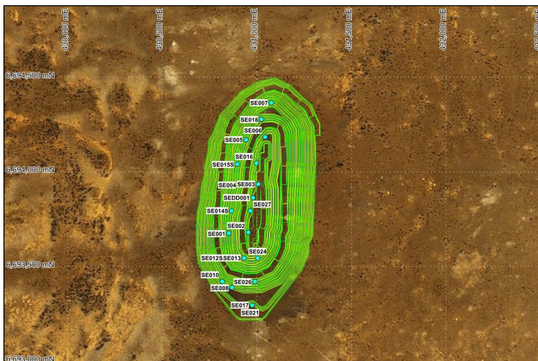
Figure 2: Sequoia drill hole collars and pit design
