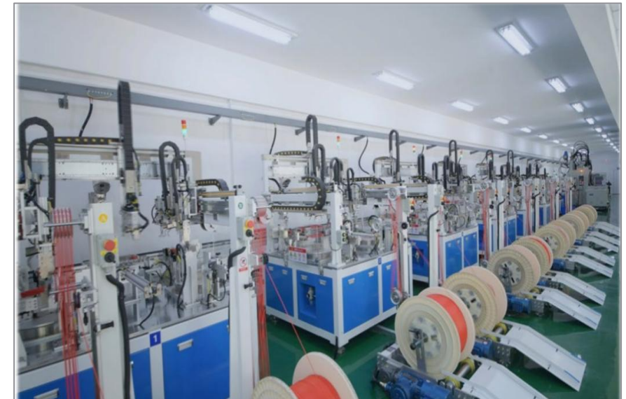
Automated Production Line for Electronic Detonators
