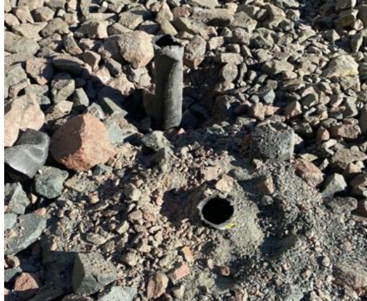
TRADITIONAL PIPING PROCESS WITH POOR OPERATIONAL AND BLAST OUTCOMES
