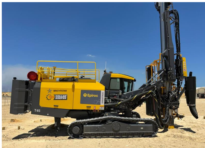
Figure 1- Aquirian's new Epiroc T45 drill and blast rig with the patented Collar Keeper fitted
