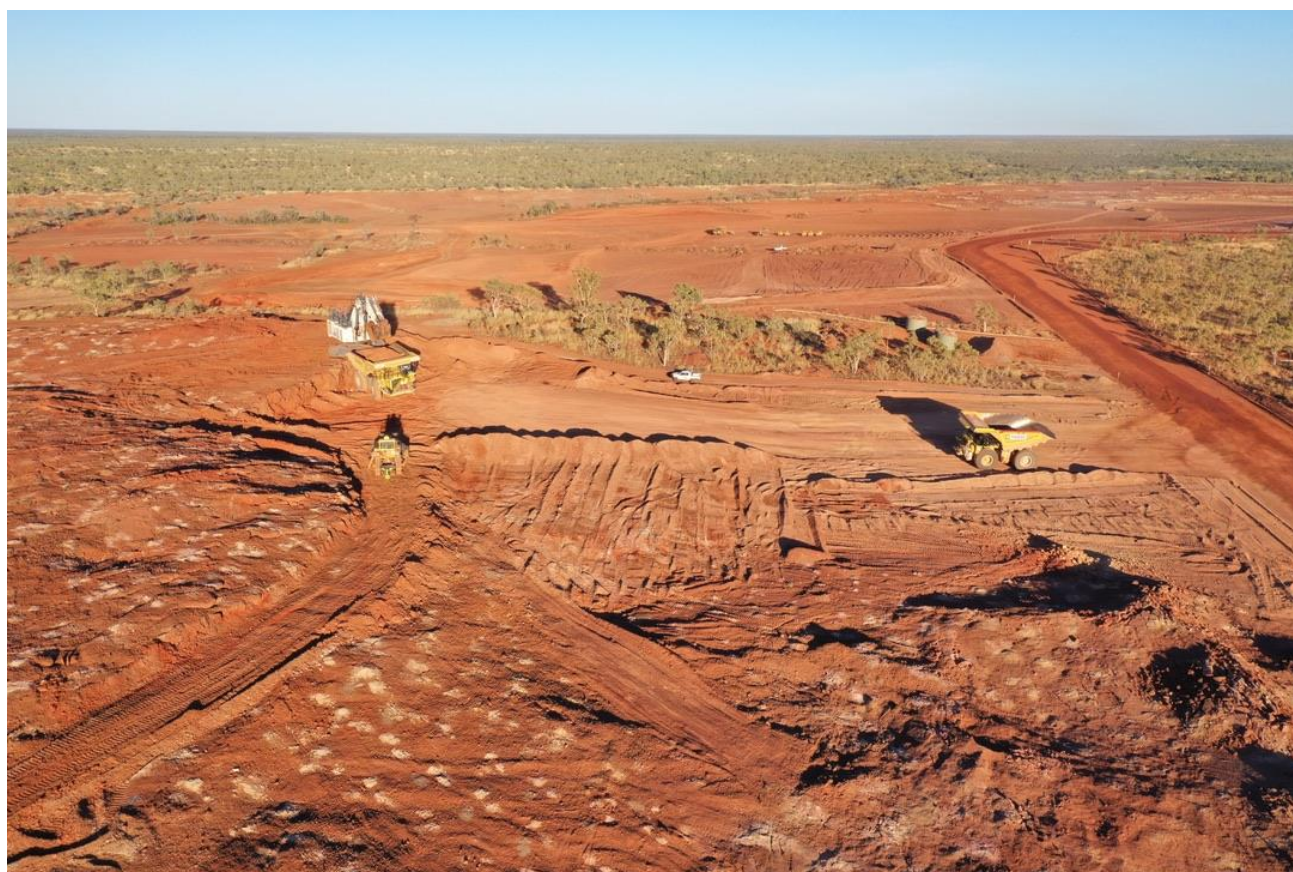
Image 9. Commencement of mining at Anthill east pit area. Clearing of pit areas, waste rock stockpile areas and topsoil stockpiles completed. Haul roads have been established.
