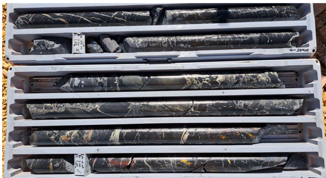
Figure 4. Diamond drill core containing sulphide copper mineralisation from drillhole MTKD010 at Flying Horse pit.
