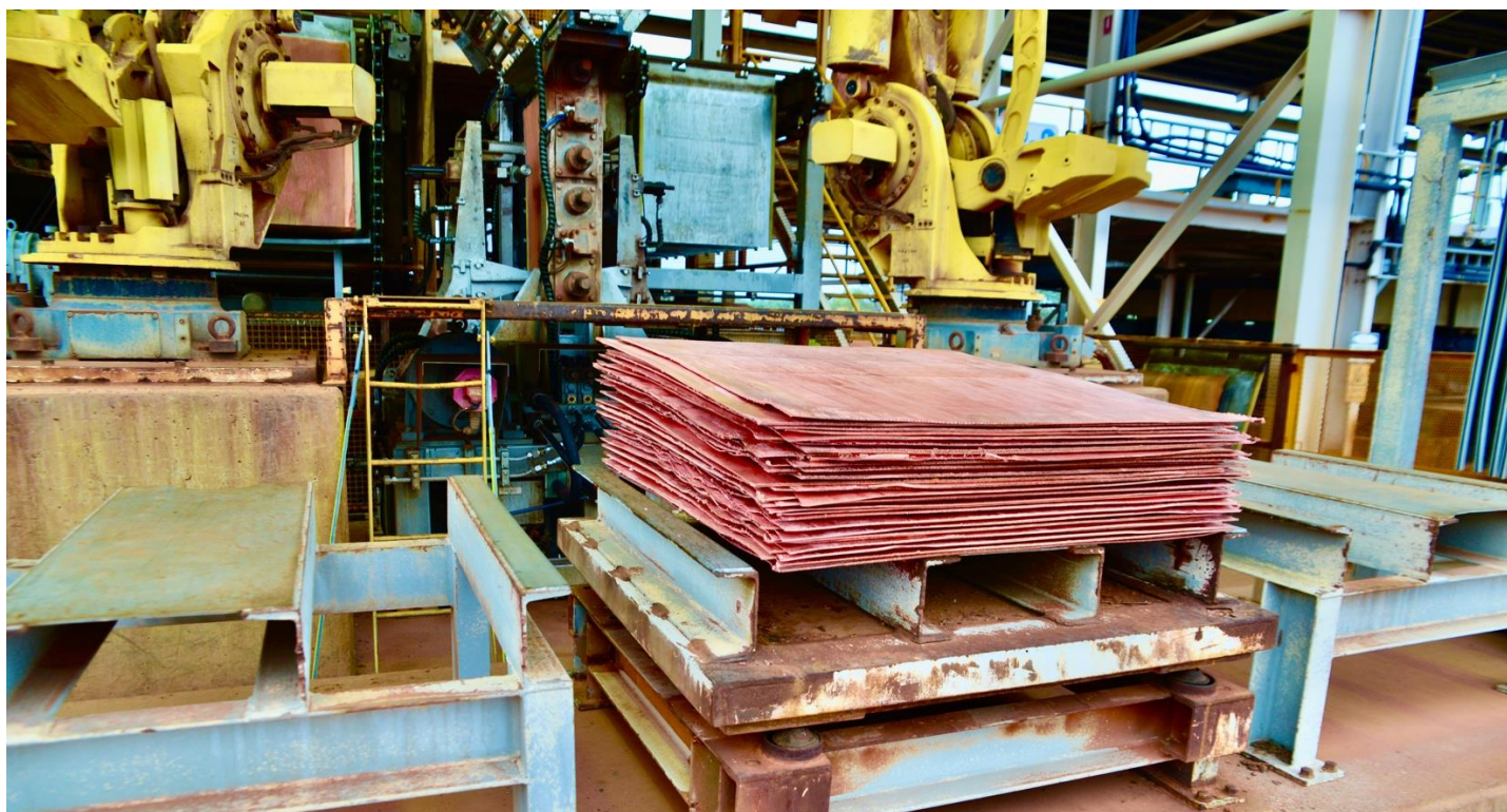
Figure 7. Stripping and stacking copper cathode sheets at the electrowinning circuit.
