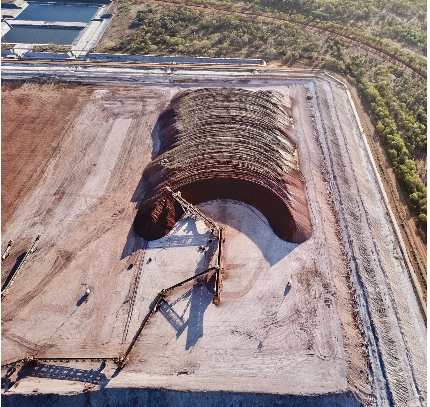
Figure 1. Ore stacking at Pad 21, Mt Kelly heap leach pad. Process ponds in background. Adjacent Pads 19 and 20 to left hand side are ready to accept ore.
